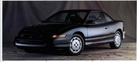
The SC features a sport-tuned suspension system with front and rear stabilizer bars, as well as a strut-valving system tuned for better performance handling.
