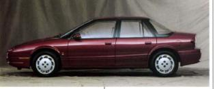
The SL2 is styled a little differently than the SL1. It features body-colored bumpers and door handles, a rear reflector panel, and fifteen-inch alloy wheels.
